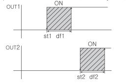
(2) DIP(Linked type) Linked control of OUT1, OUT2 by ST1, ST2(ST1 + ST2)
