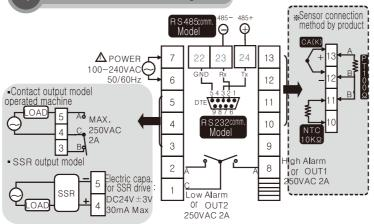
\*\* Relay connection capacity is less than 250VAC 2A. If you use the load beyond contact capacity, it will lead to contact deposition, contact failure or relay damage
