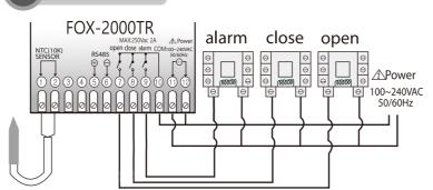
\*\* The capacity of relay connection is below 250VAC 10A. Be careful as using the load exceeding the capacity of the junction may cause bonding of the junction, contact failure, breakage of the relay and etc.
